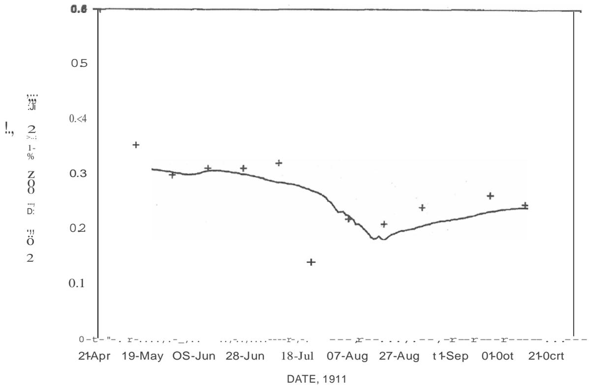
Fig. 4. Comparison between the estimated ( - ) and the fortnightly measured moisture contents ( + ) at a depth of 75 cm (IC,) for profile No. 18.
